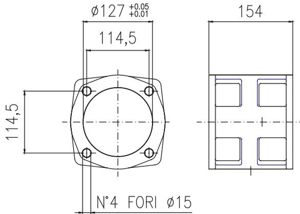
CONNECTION KIT > KIT CONEXIONES > ANSCHLUSS KIT > KIT CONNESSIONI > KIT DE CONNEXIONS
