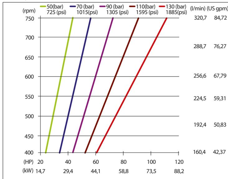
> Performances refer to theoretical delivery with 100% volumetric efficiency. For continuous or heavy-duty use, contact our technical department
