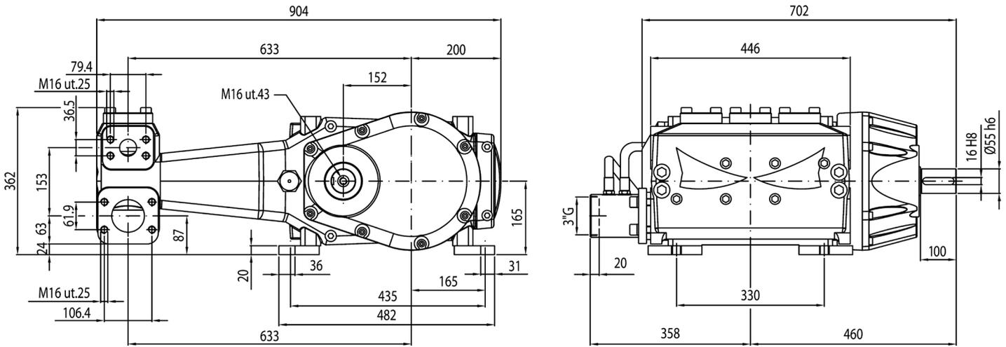
GEARBOX MOUNTING POSITIONS > POSICIONES DE MONTAJE REDUCTOR > MONTAGEPOSITIONEN UNTERSETZUNGSGETRIEBE >
