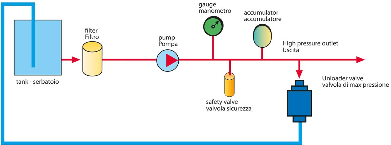
INSTALLATION SCHEME With pressure relief valve
