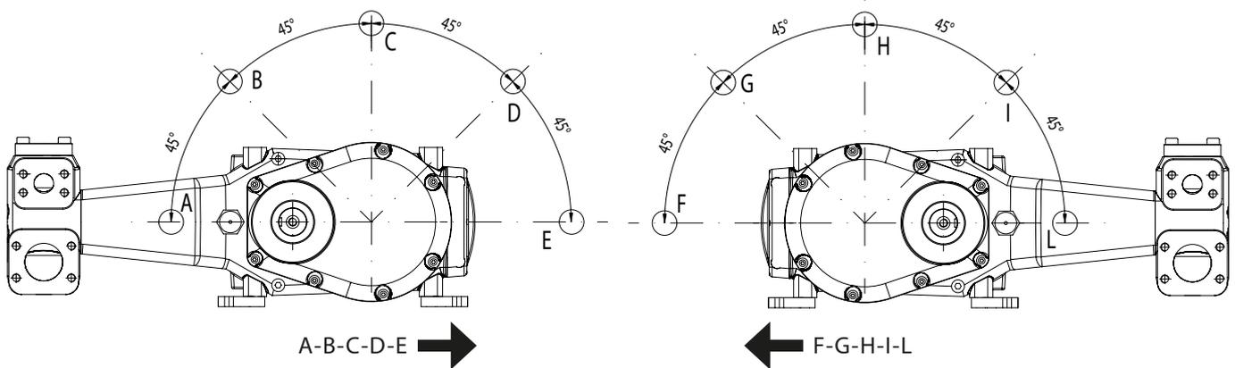
CONNECTION KIT > KIT CONEXIONES > ANSCHLUSS KIT > KIT CONNESSIONI > KIT DE CONNEXIONS
