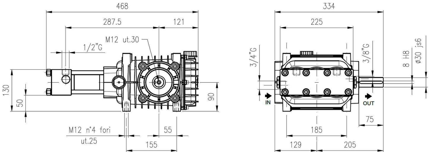
HYDRAULIC MOTOR FLANGE > BRIDA MOTOR HIDRÁULICO > FLANSCH HYDRAULIKMOTOR > FLANGIA MOTORE IDRAULICO > BRIDE MOTEUR HYDRAULIQUE
