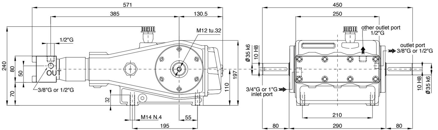
HYDRAULIC MOTOR FLANGE > BRIDA MOTOR HIDRÁULICO > FLANSCH HYDRAULIKMOTOR > FLANGIA MOTORE IDRAULICO > BRIDE MOTEUR HYDRAULIQUE
