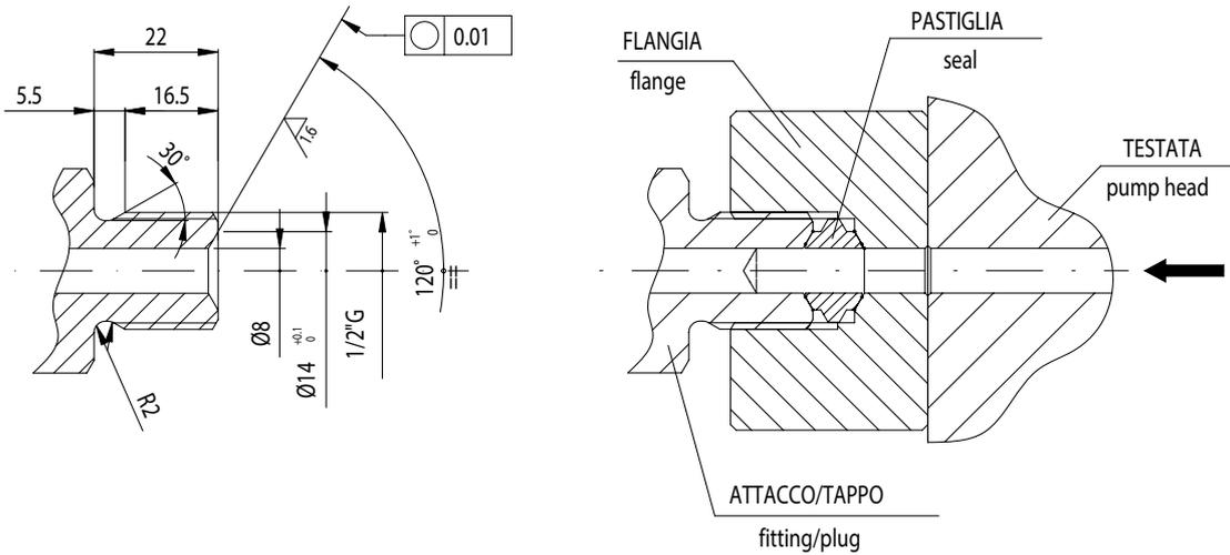
CONNECTION KIT > KIT CONEXIONES > ANSCHLUSS KIT > KIT CONNESSIONI > KIT DE CONNEXIONS
